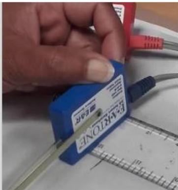
Figure 1. Placement of magnetic field probe over body of Eartone 3a insert.
